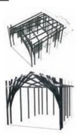
the limited space; the structure provided shelf space and hanging space for products and garments thus providing an increased display area in a small space. This structure was created with the intention of reuse with the rearranging of parts of the wooden structure in different spaces as per requirement. The parts of the structure are presently in use inside the retail store of Arch.
