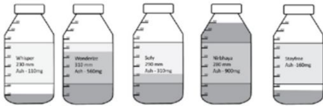
quantities of ash produced on burning different brands
